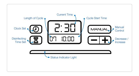
Your SoClean timer will allow you to completely automate your daily cleaning. The SoClean comes preset to start a 7 minute cleaning cycle at 10:00 am. First set the clock to match your current time. You can easily change these settings by following the steps on the next pages.
