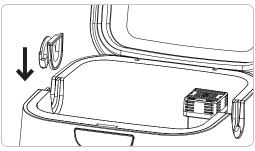
2. Install the removable hose slot plug into one open slot.
