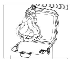
3. Insert your mask into the chamber allowing its attached hose to rest in the open hose slot.
