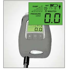
The Z1 can be removed from the PowerShell by pressing the two () icons on the sides of the PowerShell and sliding the Z1 out.
