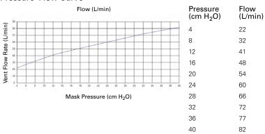
**Note:** The mask contains passive venting that meets the requirements for protection against rebreathing as specified in ISO 17510-2. As a result of manufacturing variations, the vent flow rate may vary.
