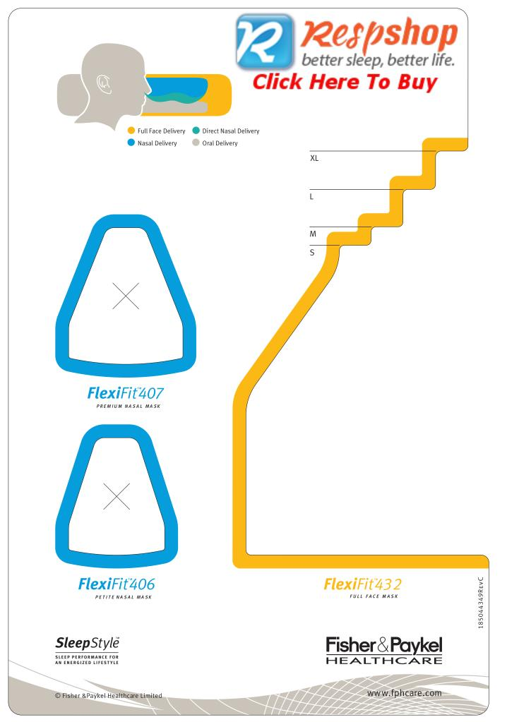
SIZE: 180 mm x 265 mm CORNERS: 5 mm & 2 mm radius COLOUR: Black, Blue 299C, Green 7473C, Warm Grey 4 Orange 130 Legend on Clear Material Background MATERIAL: Polypropylene 0.8mm CLR Rhino (Sand/Sand Finish)
