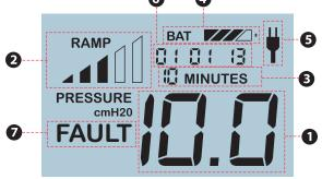
If dR-R DFF appears in the general status display, the internal battery needs replacement, so the device has stopped logging data. Call Breas to arrange for the battery to be replaced. Until then therapy will continue to be provided.
