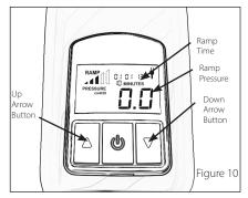
repeatedly press either the *Up* or *Down Arrow Buttons* to increase or decrease the ramp time in 5 minute increments. (Figure 10) Set the ramp time to "00 MINUTES" to disable the Ramp Mode.
