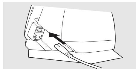
**2** Create a small loop on the cable in order to prevent stretching. Secure the power cord using the cable holder.
