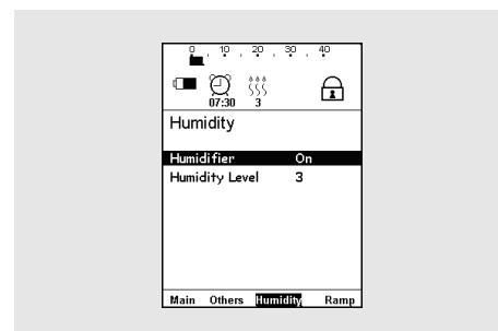
The HA 20 humidifier can be activated and deactivated by pressing the humidifier soft key for more than 1 second.
