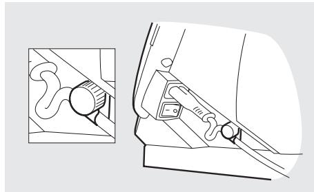
**3** Connect the power cord to the AC power source.
