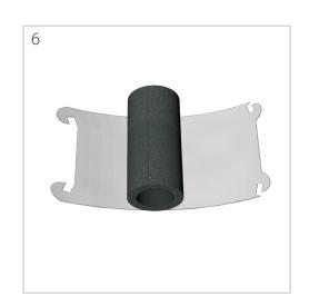
Take the new inner foam baffle material and place this on top of the plastic sleeve liner. Roll the foam material so that the edges of the plastic sleeve liner meet and the tabs are adjacent to each other. Once the tabs are aligned, slip one of the tabs past the other such that they interlock.
