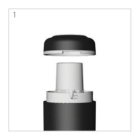
Remove the Retaining Clip of the Qtube by placing the tip of your finger in the slot (see Fig. 1) and pull away from the body of the Qtube
