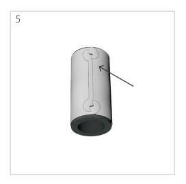
The foam baffle material will be wrapped enclosed within the plastic baffle sleeve. If you are replacing the foam baffle material disengage the locking tabs.
