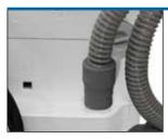
Attach tubing to air supply port on the back of the humidifier. Push rubber seal downward until it meets the plastic. **NOTE:** The rubber air supply port plug should be sealing the port on the back of the CPAP, not the port on the bottom of the unit.
