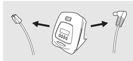
**5** Clean the outside of the iSleep 20 using a lint-free cloth and a mild detergent solution. If the iSleep 20 needs to be disinfected, this can be done with Virkon® or Lysetol® Med.
