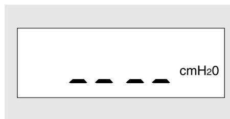
In order to start the treatment again, start to breath in the mask or press the Start/Stop button shortly. The iSleep 20 will then increase the pressure to the set level during up to 10 seconds.
