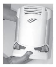
3. Insert the AC or DC power supply into the power port receptacle on the front, bottom right side of the unit.
