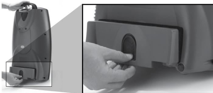
To remove the Battery, pull down on the black release lever. While holding DOWN the release lever, pull the Battery away from the Eclipse 5.
