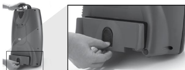
When the battery is properly installed and the Eclipse 5 is ON, the Power Cartridge Status Gauge
