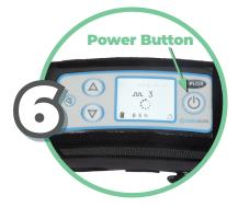
Turn on the X-PLOR by pressing the power button for 2 seconds. Set the flow setting to your prescribed setting and use normally.
