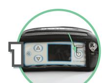
Turn off the X-PLOR® by pressing the power button for 2 seconds.
