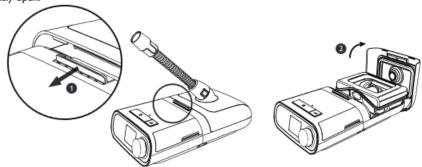
3. Remove the tank (1) by grabbing both sides of tank and lifting out of the humidifier base. Rinse the tank with water. Place the tank on a firm, flat surface. Fill the tank with water (2) no higher than the maximum fill line ( ). To avoid spilling, the water level should not rise above the bottom of the tube (3) in the back of the water tank.
