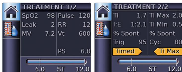
The intuitive treatment screen displays the patient's inspiratory and expiratory pressures in an easy-to-read bar graph, in addition to other patient data such as minute volume, tidal volume, inspiratory time, I:E ratio, leak and respiratory rate at every breath.
