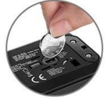
Open the fuse's cap with a coin or similar thin item
