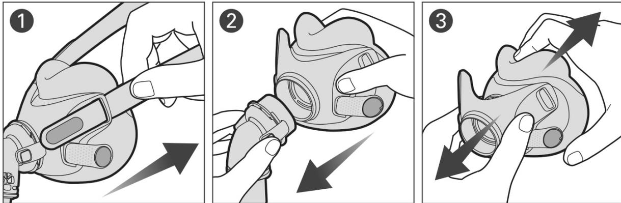
1. Undo the fastening tabs on the upper headgear straps and pull them from the frame. Keep the magnetic clips attached to the lower headgear straps.
