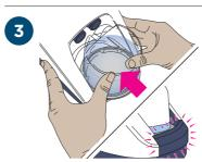
Fit the water chamber onto your device by depressing the finger guard, pushing forward until the finger guard clicks into place.
