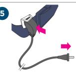
Plug myAIRVO 2's power cord into the mains/utility power socket and into the rear of the unit.
